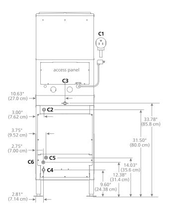
Measurements shown are with base stand legs at lowest position.
